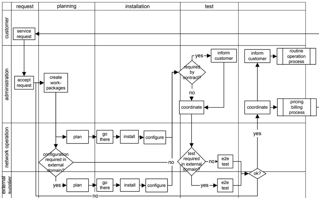
Fig. 3: Activity-based description of service provisioning process
