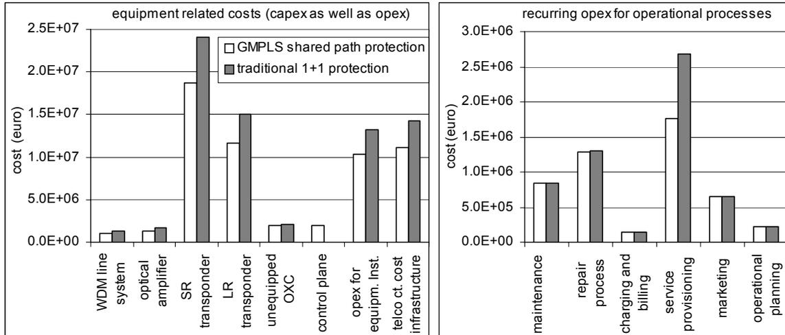
Fig. 4: CapEx and OpEx costs for German reference network scenario.
