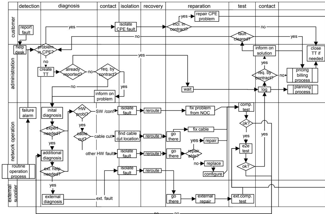
Fig. 2: Activity-based description of repair process
